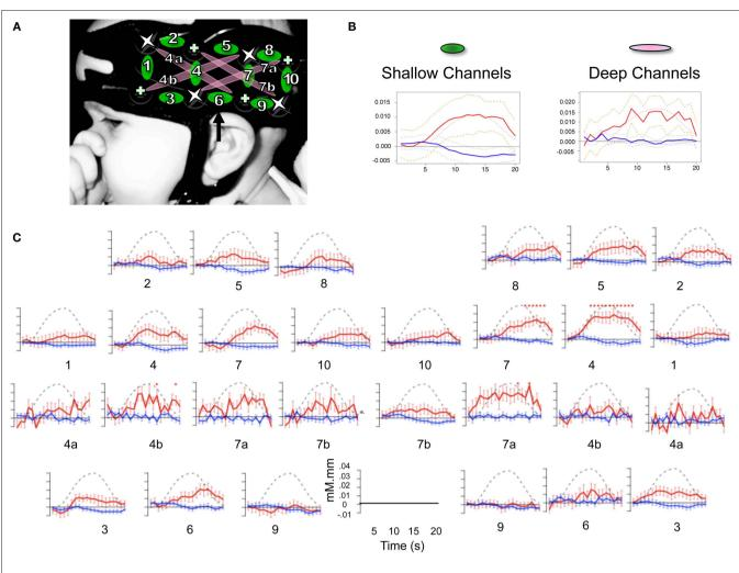
**FIGURE 2 | (A)** Design of the probe array showing distribution and separation of sources and detectors. Location of the 10 shallow channels (1–10) and 4 deep ones (4a,b and 7a,b) on an infant's head. Crosses indicate detectors and stars sources. Channel 6 is aligned to the T3 position in the international 10–20 system. **(B)** Time course of Hb changes averaged over
