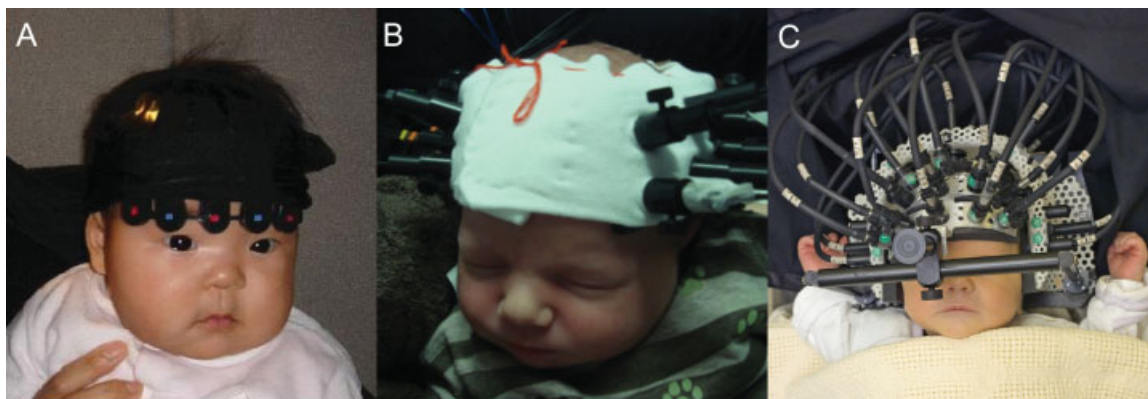
Figure 3 The NIRS measurements of (A) frontal activation in a 3-month-old infant using a Hitachi CW optical topography system, (B) temporal activation in a newborn infant using the UCL CW optical topography system, and (C) 3D optical properties of a newborn infant brain with the UCL time-resolved optical tomography system.
