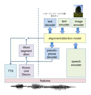
Fig. 1. Functional blocks of the "Speaking Rosetta" project
